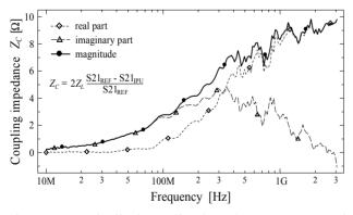
Figure 7: Longitudinal coupling impedance  $Z_C$  measured with a coaxial setup of  $Z_L = 50 \Omega$  (wire method). For the S21<sub>REF</sub> reference measurement the IPU was replaced by an equivalent length of a straight tube.
