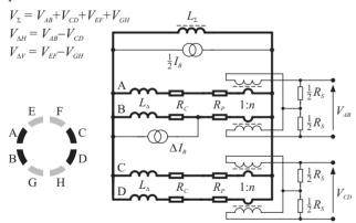
Figure 4: IPU low frequency model for one plane.
