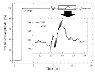
Figure 8: IPU TDR measurement with a 50  $\Omega$  coaxial setup (wire method) and TDR module Agilent 54753A. Ripples in the magnified region originate in setup waveguide modes and the irregularities outside the region result from setup imperfections, especially of the conical adaptations.
