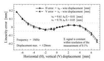
Figure 6: IPU linearity error. Measured with a wire of diameter of 0.2 mm displaced diagonally.
