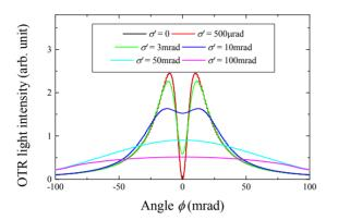
Figure 2: OTR angular pattern for different values of beam divergence
