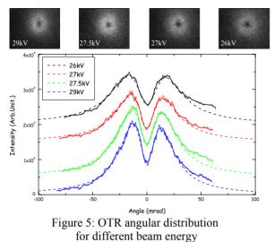
The results, summarized in table 1, show that the agreement between spectrometer and OTR measurements is very good for the two first voltage values. A discrepancy of 10% is then observed, possibly due to aberrations in the optical system or a misalignment of the electron beam entering the spectrometer line, which is very sensitive for energy measurements.
