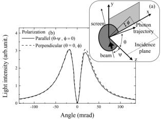
Figure 1: (a) Geometrical configuration: The incident plane contains both the normal to the screen and the beam velocity (b) OTR angular distribution,  $I_{//}$  and  $I_{\perp}$  for a 50MeV electron. The tilt of the screen introduced an asymmetry of the lobes pattern, only visible in the  $I_{//}$  signal. The relative position of the maximums with respect to the centre of the distribution gives a measurement of the beam energy (=1/ $\gamma$ ).
