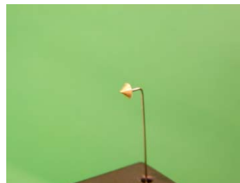
Figure 7: Photograph of the opaque disk to block the glare of central image.
