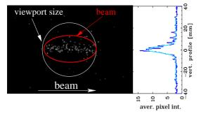
Figure 2: The two dimensional image from the intensifier of a Ar<sup>10+</sup> beam at 4.7 MeV/u and  $I_{beam} = 2.5$  mA recorded during *one* 250  $\mu$ s long macro-pulse with a vacuum pressure of about 10<sup>-5</sup> mbar and the projection for the vertical beam profile (right) are shown [6].
