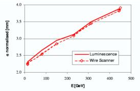
Figure 4: Comparison of the normalized vertical profile width as determined by the BIF-method and a flying wire scanner at CERN-SPS [7].
