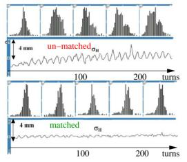
Figure 9: Horizontal beam evolution on a turn-by-turn basis and the associated rms beam width for an un-matched and matched case [10].
