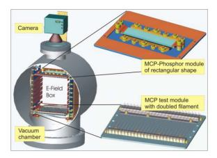
Figure 6: Schematic sketch of an IPM.
