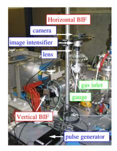
Figure 1: The installation of BIF station at GSI [6].
