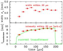
Figure 3: The width variation during a macro-pulse of 8 mA  $Ar^{10+}$  at 11 MeV/u is shown. The lower graph compares the normalized image intensity with the beam current [6].
