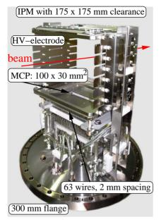
Figure 7: Photo of the IPM at the GSI synchrotron [15].
