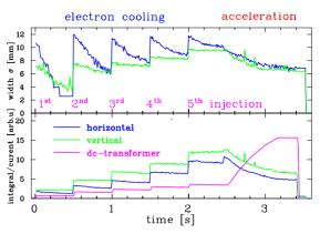
Figure 8: The process of beam stacking by electron cooling of a 11.4 MeV/u U<sup>73+</sup> beam during 5 injections followed by an acceleration to 400 MeV/u at the GSI synchrotron is monitored. The horizontal and vertical beam width  $\sigma$ during the 3.4 s long cycle is shown on top and the integral of the individual profiles as well as the dc-transformer on bottom. Each 10 ms a profile is recorded [15].
