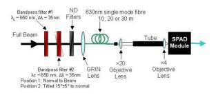
Figure 2: Optical arrangement employed to couple the synchrotron beam into the  $4.3\mu m$  core fibre (single mode at a wavelength of 630nm) and optically image the photons onto the  $50\mu m$  diameter SPAD.
