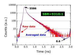
Figure 4: Histogram taken using the setup in Figure 2 employing two BP filters and 10m of Single mode fibre
