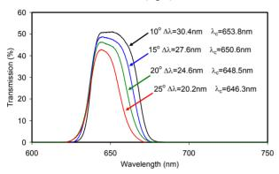
Figure 1: Transmission spectra of two bandpass filters in series, one placed at normal incidence and the other at  $10^{\circ}$ ,  $15^{\circ}$ ,  $20^{\circ}$  or  $25^{\circ}$  to the normal.
