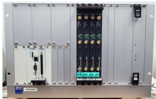
Figure 3: 6U PXI crate from EKF with a 3U NI controller and four 6U Acqiris DC241 digitizer modules
