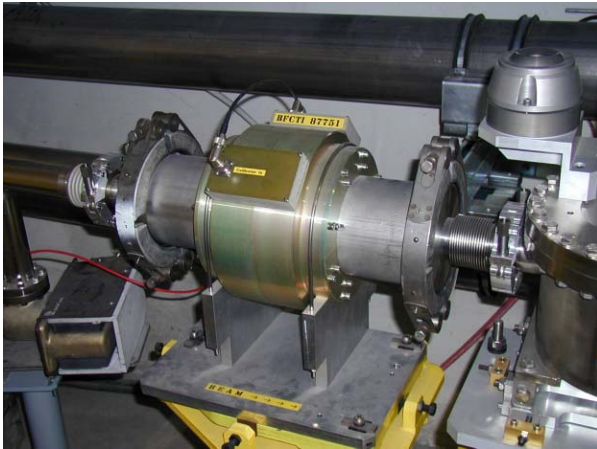
Figure 3: A Fast BCT device on the TI8 line.
