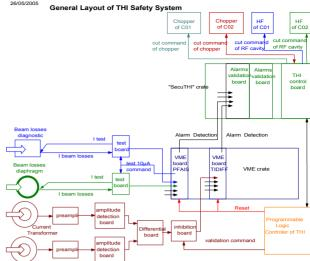
"Alarm detection" signals are generated by VME boards and sent to "alarm validation" boards. "THI control" board collects all alarm signals. A programmable logic controller indicates to the control board different configuration states. If "surveillance" mode is validated for example, when a VME board generates an alarm detection, the THI control board commands the chopper to cut the beam. If a problem is detected on the chopper, the acceleration voltage of the C0 injector is cut.
