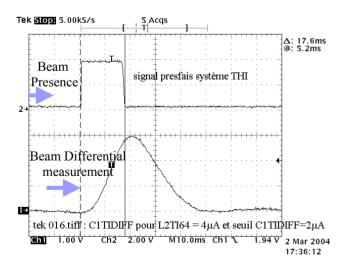
The response time for a beam current of  $4\mu A$  and a threshold of  $2\mu A$  is around 18 ms. It depends of the ratio between threshold and loss current.
