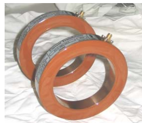
Figure 3: Picture of 2 Fast Current Transformers BERGOZ FCT-082-10:1-WB
