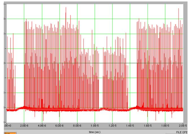
Figure 14 Wall current monitor of all 100 bunches. The first 50 were cooled for two hours.
