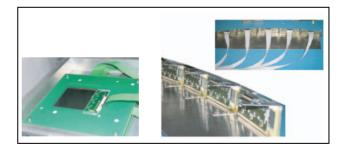
Figure 2: Left: silicon micro-strip chambers, acting as active target for bremsstrahlung; right: silicon micro-strip tagging modules.
