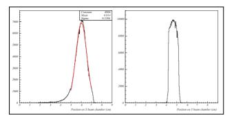
Figure 6: Impact point of the incoming electrons in the horizontal and vertical coordinates measured by the target silicon micro-strip planes (energy of incoming electrons of 424 MeV).
