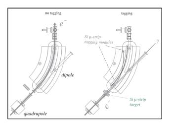
Figure 1: Left: layout of the final part of the BTF beamline; the electron beam can exit either from the straight section (bending off), or from the  $45^{\circ}$  curved section (bending on). **Right:** layout of the photon tagging; the electron irradiates a bremsstrahlung photon on the silicon micro-strip target, and impinges on one of the 10 silicon micro-strip tagging modules outside the wall of the curved section of the beam-pipe.
