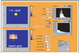
Figure 8: Online panel of the triple-GEM pads readout, showing the beam profile for one electron peak (top) or for the total beam spot (bottom).
