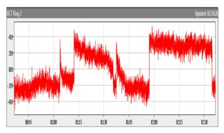
Figure 6 : First circulating beam in ring 2 seen by BCTDC A (12/9/2008).
