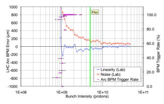
Figure 3 : BPM auto-trigger threshold determination – HIGH sensitivity mode (10/8/2008).
