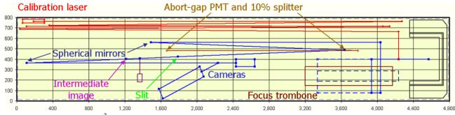
Figure 3: A new 4.8×0.8 m<sup>2</sup> optical table below the beam adds a calibration path and focus trombone. Light enters at right.
