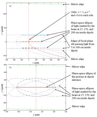
Figure 2: (a) Horizontal and (b) vertical phase space for emission in D3, with the coordinates and the optical focus in middle of the path selected by the slit.
