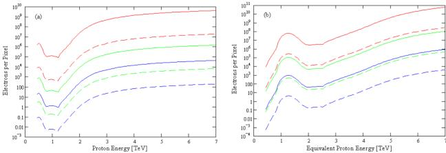
Figure 4: Electrons in the peak pixel of the camera in one turn (dashed curves) and in a 20-ms video interval (solid curves); for a pilot bunch (blue), a single full bunch (green), and a full ring (red). (a) Protons and (b) lead ions.
