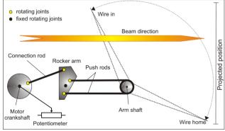
Figure 4: Schematic of a wire movement.
