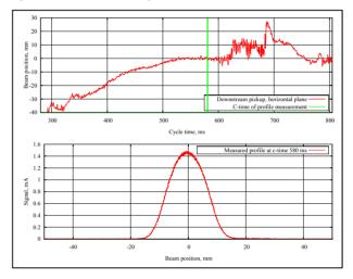
Figure 8: Horizontal profile measurement of a c entred beam in the PS booster: a) beam position from a downstream pickup, b) profile, measured by a wire scanner.
