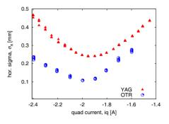
Figure 5: Hor beam sizes during a quad scan, inferred after analysis of the YAG and OTR images (MBM, 4 nC).
