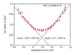
Figure 2: Beam size decreases linearly as we approach the beam waist (approximately at -1.8 A). Below 0.28 mm, the beam size enters a saturation regime. The blue line shows two linear fits to the data at each branch, and stresses the lack of linearity between -1.7 A and -1.9 A, which points the YAG saturation.
