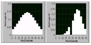
Figure 3: Beam profile left: profile x, right: profile y.
