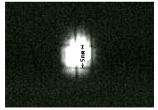
Figure 6: Beam profile (C6+, 200MeV/u).
