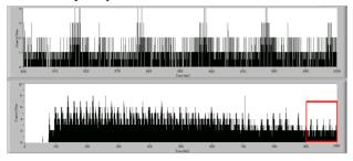
Figure 4: Spill structure (zoomed and total) measured by scintilator (sampling rate is 100 kHz, C6+, 200 MeV/u).
