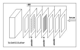
Figure 2: Structure of detector in pocket.
