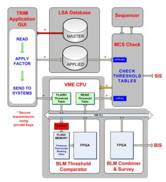
Figure 2: Block diagram of the data flow for the parameters configuration and verification.
