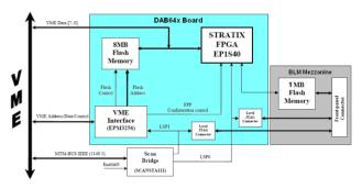
Figure 1: Block diagram of the FPGA firmware deployment and initialisation options.
