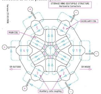
Figure 3: Layout of the auxiliary correctors in a sextupole.
