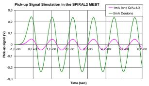
Figure 3: MEBT Pick-up Signal Simulation.
