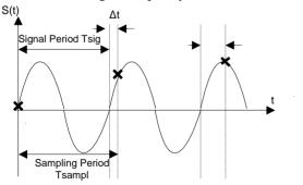
Figure 6: Under-sampling Timing.
