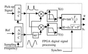
Figure 7: I/Q Diagram.
