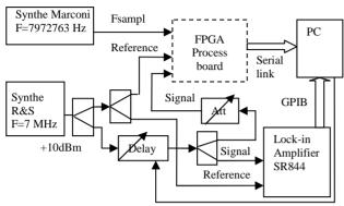
Figure 9: Test Bench Diagram.
