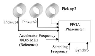
Figure 5: Assembly Scheme.
