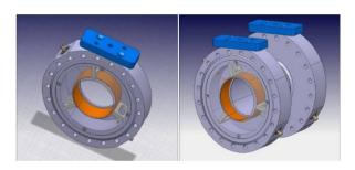
Figure 2: Pick-up Design. Diameter: 80 mm, Length: 30 mm.
