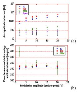
Figure 7: Average induced current (a) and phase (b) versus different modulation amplitudes. Data are collected from the LHC point 8 right and straight section including spare channels.
