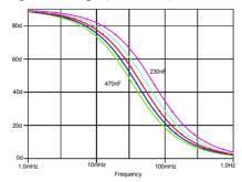
Figure 5: Phase of the Bode diagram for different values of  $C_{\rm filter}$ .
