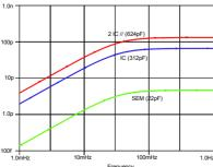
Figure 4: Magnitude of the Bode diagram for the 3 monitor types (SEM, IC and IC2).
