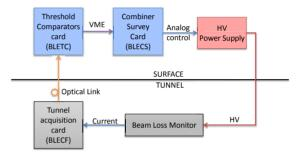
Figure 2: The LHC BLM system looped for the connectivity test.
