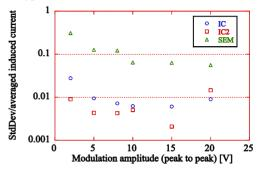
Figure 8: Measurement reproducibility versus modulation amplitude. Different options are being investigated to reduce the SEM error.
