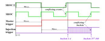
Figure 3: Schematics of various clocks generated by the EVG. See text.
