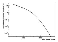
Figure 4: Simulated sublimation of the wire material in the wire center during scans with decreasing velocity.
