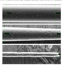
Figure 2: Fiber fracture at three distances from the beam impact location: 1 mm (upper plot), 0.5 mm (middle plot) and at beam center location (bottom plot).
