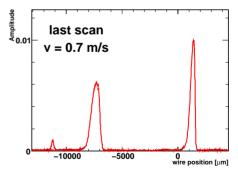
Figure 1: The last profiles after which the wire has been found broken. Upper plot shows breakage of vertical wire: deviations from Gaussian profile are visible. The bottom plot shows breakage of the horizontal wire: multiple peaks suggest that the wire has already fragmented.
