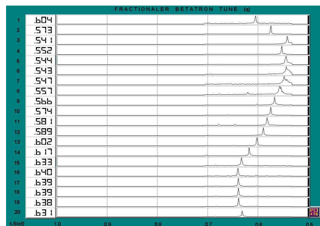
Figure 3: Display of a tune measurement in the ramp consisting of averaged FFT spectra
