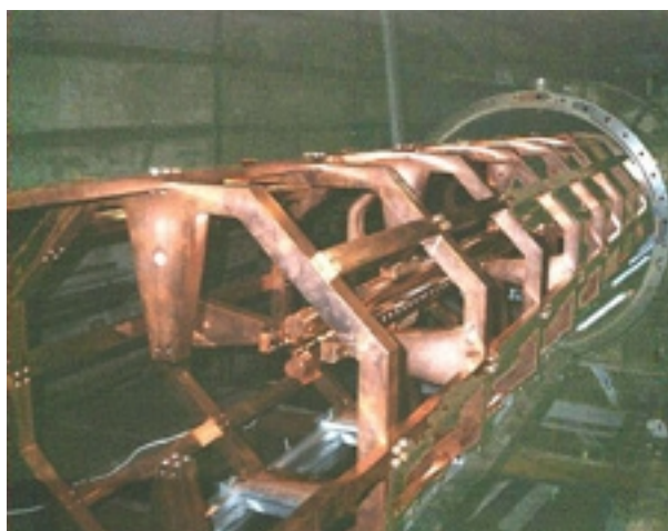
Figure 1: View of the RFQ structure at the assembling place.
