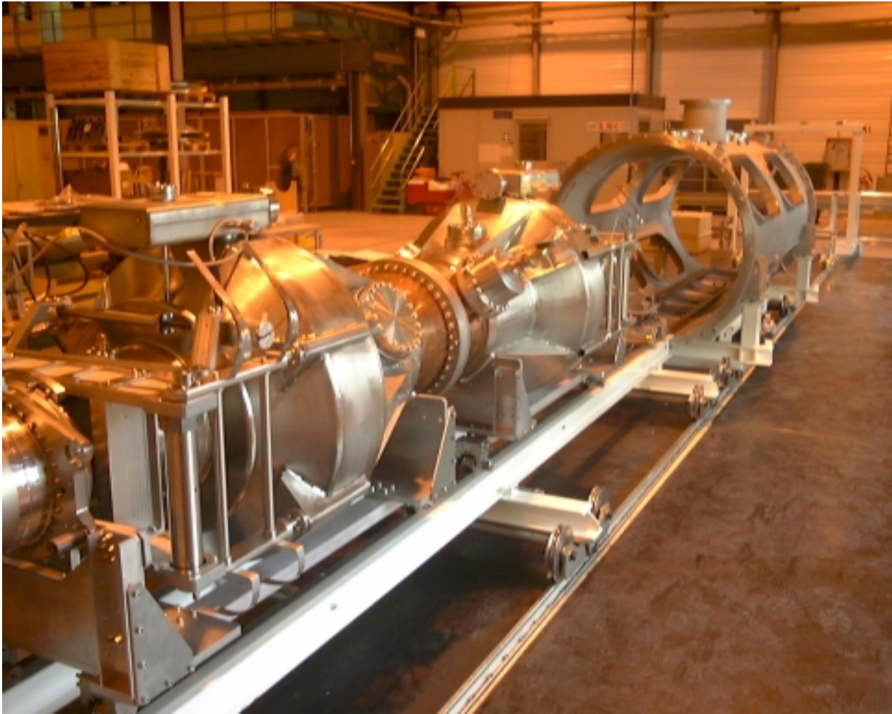
Figure 1: Assembly of the SOLEIL cryomodule at CERN
