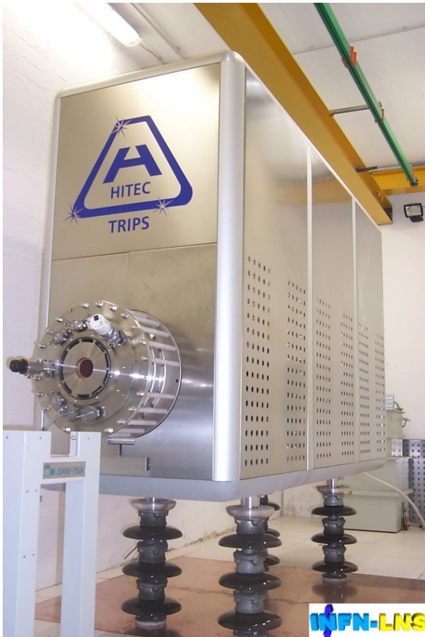
Figure 7: The 100 kV high voltage platform.
