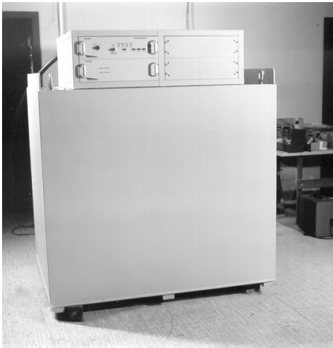
Figure 4: PowerMod™ HVPM 140-500 modulator with controls. (approximately 4' x 5' x 6')
