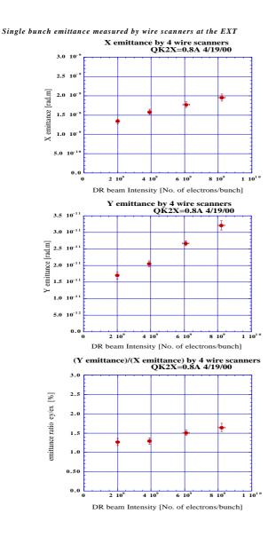
Figure 2: Recent results of emittance measurements using wire scanners at the EXT.
