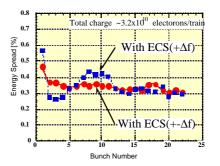
The single-bunch energy spread was less than 0.5% expect for first bunch at the case of total charge/pulse= $3.2 \times 10^{10}$ . The single-bunch energy spread was generated by a RF slope in ECS structures was not observed in these intensity.
