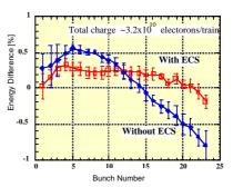
After the adjustments of the ECS RF phase, the RF power of the K1ystrons were set to get a flat energy distribution for all bunches with 1.9MW for +  $\Delta f$  and 1.5MW for - $\Delta f$ . The a BPM miss-reading by the beam loss of the collimator in front of the BPM.
