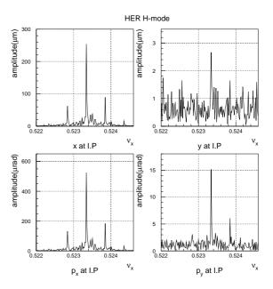
Figure 3: Typical spectrum of FFT analysis of beam oscillations at I.P in the electron ring(HER). The phase spaces are reconstructed by two OctoPos data using transfer matrices between OctoPos and I.P. The beam oscillations are excited by a shaker in the horizontal plane(H-mode).
