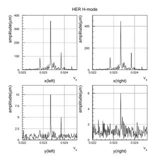
Figure 2: Typical spectrum of FFT analysis of beam oscillations at the left and right side of OctoPos in the electron ring(HER). The beam oscillations are excited by a shaker in the horizontal plane(H-mode).
