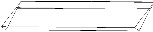
Figure 3: Model 1 geometry used for HFSS: only 1/36 of the structure is simulated. The inner and outer radii of the ferrite are 20 mm and 80 mm, respectively. The axial length is 1 m. The current sources are on the axis.
