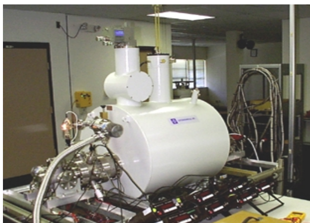
Figure 2: Picture of the NASA HiPAT trap designed to transport 10^{12} antiprotons.
