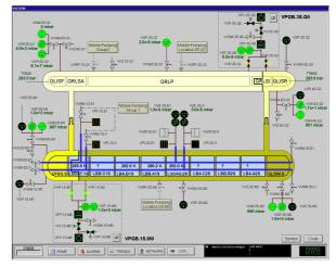
Figure 2: The Vacuum synoptic showing the String2 sketch.
