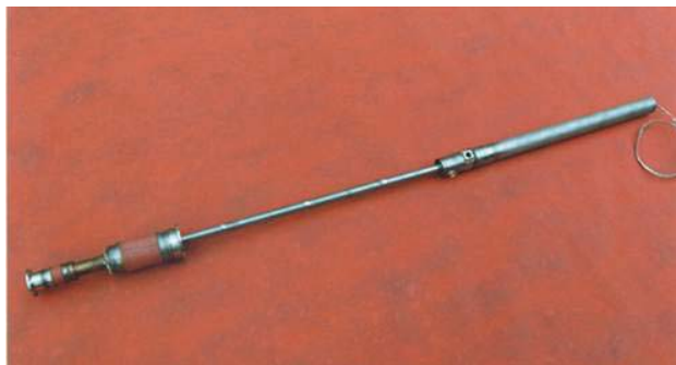
Fig. 1. Overall view of 600 A HTS current lead.
