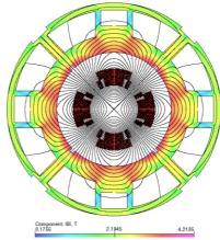
Figure 1: Optimized 90-mm quadrupole cross-section.
