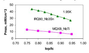
Figure 4: Quench limits for Nb3Sn IRQ and NbTi MQXB (inner-layer midplane turns) versus the critical current margin at Top=1.95 K.
