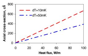
Figure 6: Total cold mass axial heat transport crosssectional area versus total cold mass heat flux.
