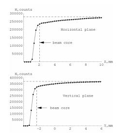
Fig.3. Beam emittance measurements with scraper. The coordinates are the scraper position and the number of counts on a scintillator. The beam core (containing 85%
