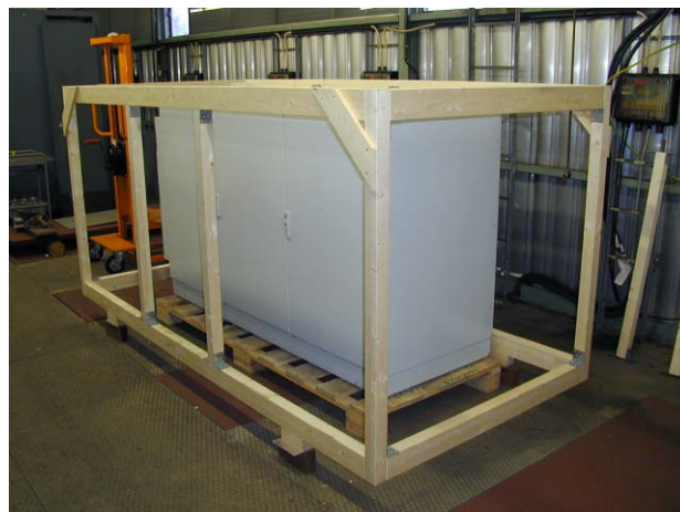
Fig. 2 Electronic rack with wooden mock up
