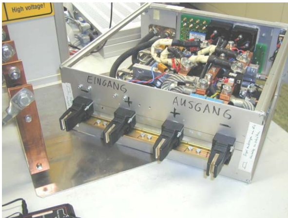
Fig. 4: Buck converter with fast connectors
