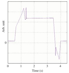
Figure 3: The voltage pattern of the focusing quadrupole magnet power supply. The horizontal betatron tune should be close to half integer at the beginning of the beam extraction. The spike like pattern at the flat top start is caused from this operation schema.
