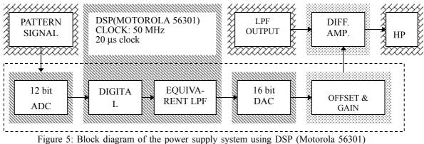
which is operated by 50 MHz, that is, 20  $\mu$ s sampling clock.
