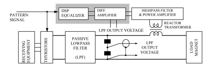
Figure 2: Block diagram of the KEK 12GeV PS main ring quadrupole magnets power supply system. Hatched parts are equalizer.
