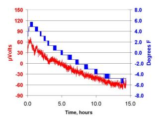
Figure 6. DAC Temperature Stability
