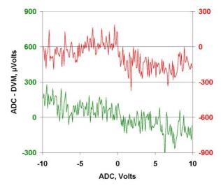
Figure 4. Linearity Results - Channels 1 and 2
