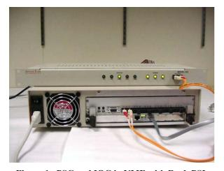
Figure 1. PSC and IOC in VME with Rack PSI
