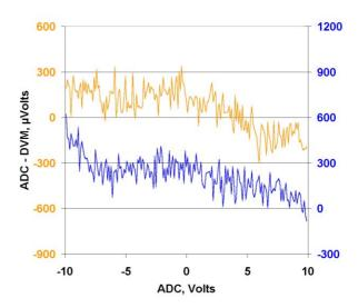
Figure 5. Linearity Results - Channels 3 and 4
