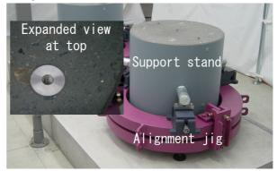
Figure 4: Full size support stand and attaching alignment jig were developed by Takenaka Co. The surface roughness and flatness are within  $\pm 10 \,\mu m$ .
