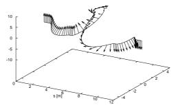
Figure 2: Orbit and spin tracking through the four helical magnets of a Siberian Snake at  $\gamma = 25$ . The spin tracking shows the reversal of the vertical polarization.
