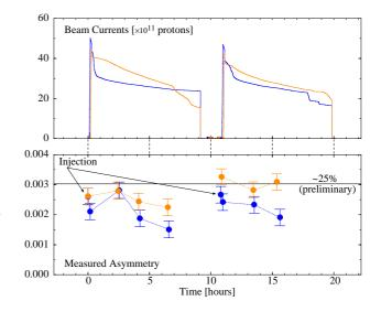
Figure 4: Circulating beam and measured asymmetry in the blue and yellow RHIC ring (blue(dark) and yellow(light) lines and symbols, respectively) for two typical stores.
