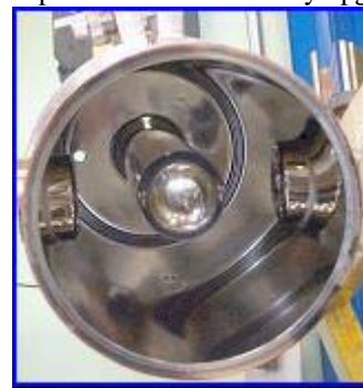
Fig. 1 Upgraded medium \beta resonators; by replacing its Pb layer with a sputtered Nb film it could reach an accelerating field exceeding 4 MV/m @ 7W dissipated power.
