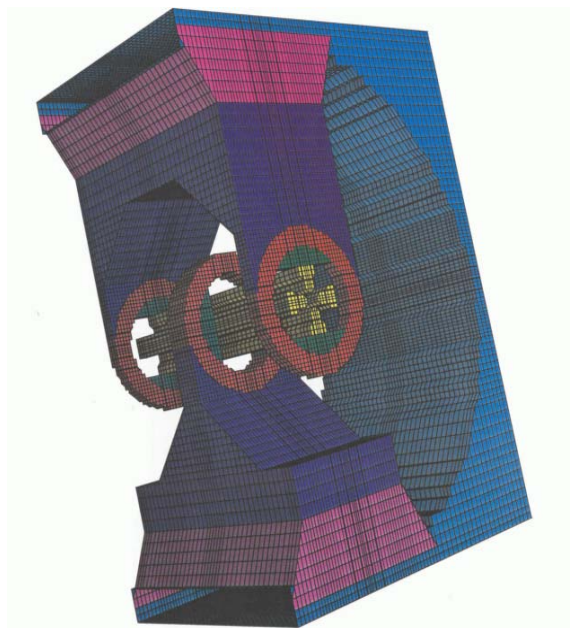
Figure 6: 3 ring slice of an IH RFQ.
