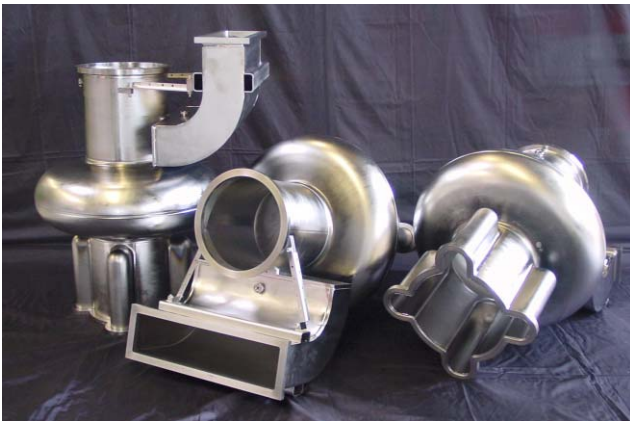
Figure 2: Three 500 MHz single cell niobium cavities ready for preparation for vertical test.
