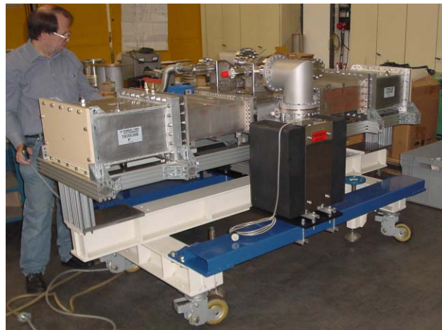
Figure 6: Two 500 MHz RF windows assembled and baked at ACCEL after final leak-check, ready for RF processing at Cornell
