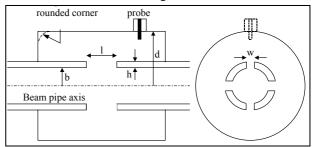
Figure 1: sketch of the bunch length monitor.
