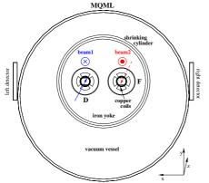
Figure 2: Cross-section of the MQML quadrupole in Q10. The magnet is (de)focusing for beam2 (beam1) in X.
