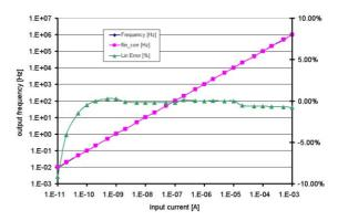
Figure 6: Output frequency of the CFC versus input current with linearity errors.
