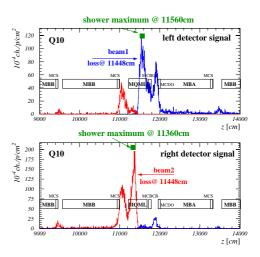
Figure 3: Simulated detector signals of shower particles, which are induced by point like losses of beam1 and beam2 in the middle of the quadrupole MQML. Top: Left detector signal along the cryostat. Bottom: Right detector signal along the cryostat.
