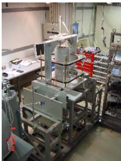
Fig.2: Measurement system of the HTS-magnetic shield and HTS-sensor. The whole system is constructed on the floor base and the position of the HTS-SQUID is controlled by the X-Y-Z stage driven by the pulse motor.
