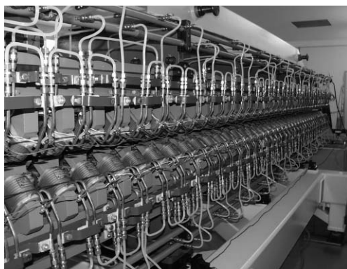
Figure 1: Side view of one UE212 section with the 4.55 m long single piece iron yoke/vertical pole structure and added horizontal poles. The inter coil connections for the two individual vertical power circuits are implemented on left or right side of each beam. The horizontal coils are attached all in series.
