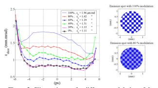
Figure 3- Slice emittance for different modulation of the densities on emission spot; r = 1mm;  $\varepsilon_{th} = 0.3$  mm.mrad.
