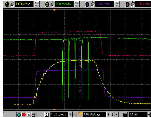
Figure 8: A burst of 5 pulses together with the RF pulses of the bunching system and accelerating cavities
