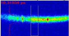
Figure 5: Streak camera picture of laser micro pulses.
