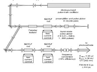
Figure 3: Optical scheme of the current PITZ laser.
